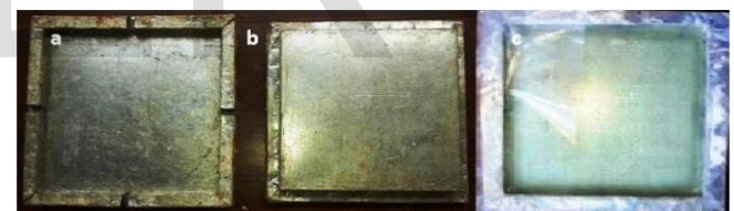
Fig. 1: (a) Bottom die used for square specimen (b) Upper die used for square specimen (c) fabricated hybrid composite specimen
